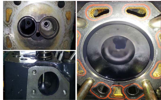
(a) Engine cylinder, Piston, Valves of Intake and Exhaust, Ports of Intake and Exhaust
