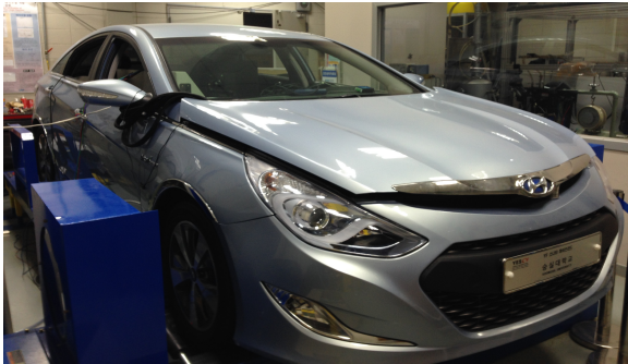
Fig. 3 TMED type parallel hybrid electric vehicle
