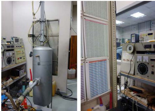
Fig. 3 Tank-pipe system to measure intake flow
